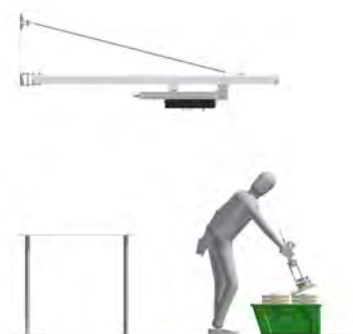
C Crane not positioned vertically above the lifted item
