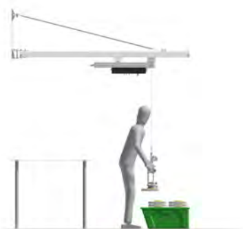
B Working too close to the lift rope
