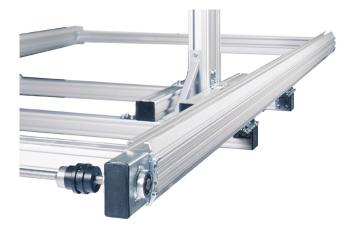
The Mechbelt is a belt driven linear unit to drive 1 or 2 or 3 axle linear movements up to a length of 14 meters in both the horizontal and vertical position. The parallel mounted units allow loads up to 500 kgs.
