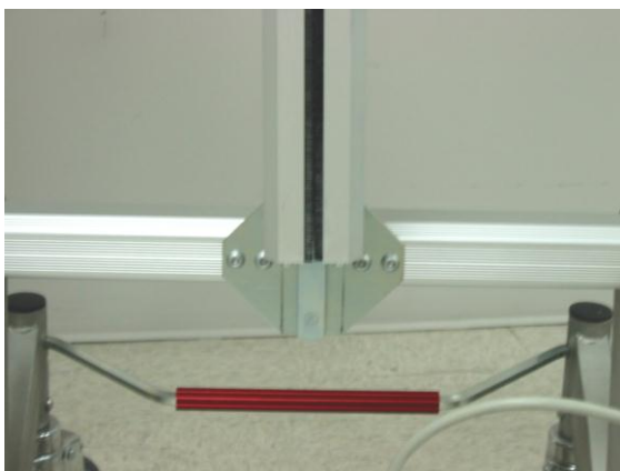
Sliding Mast into Mounting Bracket
